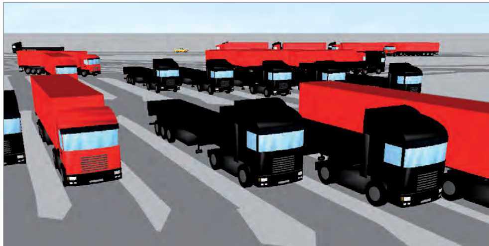
Microscopic traffic flow simulation with VISSIM to examine the planning versions for lorry dispatch
