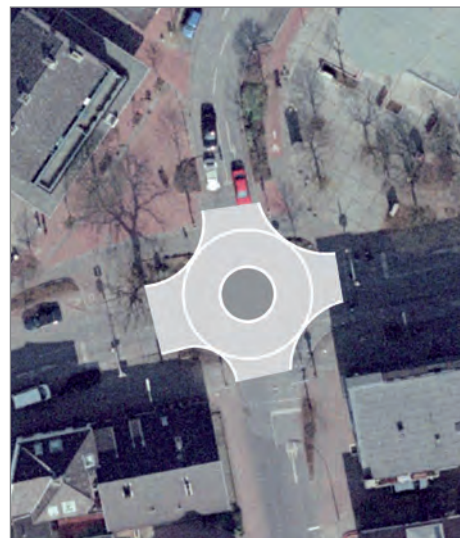
Bicycle-friendly traffic routing through the Installation of a roundabout
